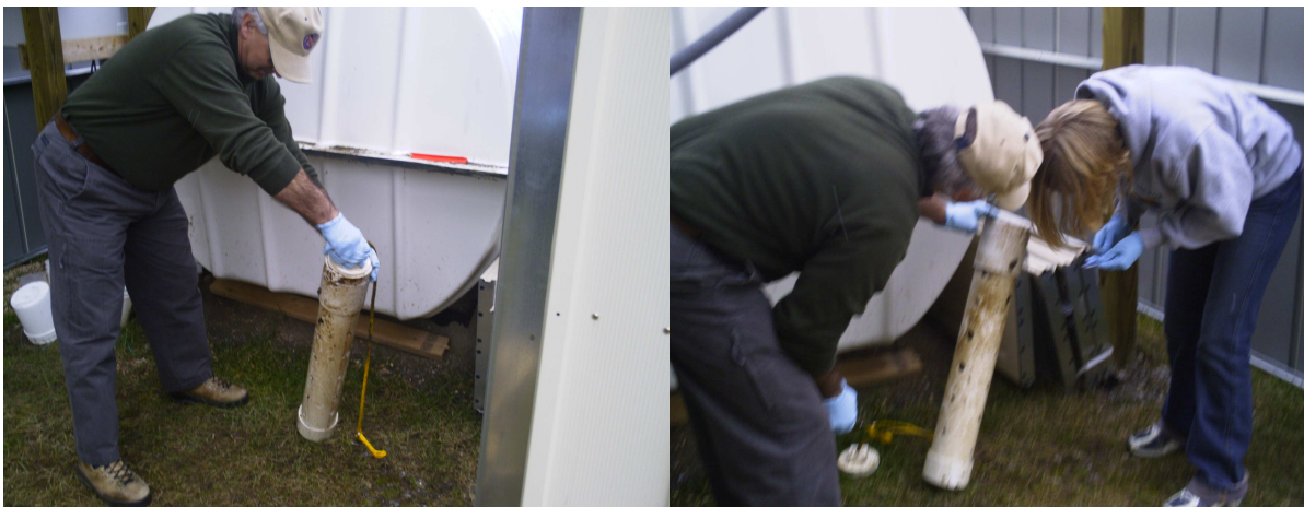
On the left, Michael Gerardi (Cromaglass microbiologist) was removing the PVC tube from SBR. On the right, Michael and I were collecting biofilm scrapings from the PVC tube and the coffee can.
