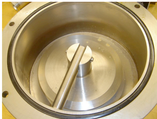
[Fig. 6c]: Open baffle valve to allow diffusion pumping.
