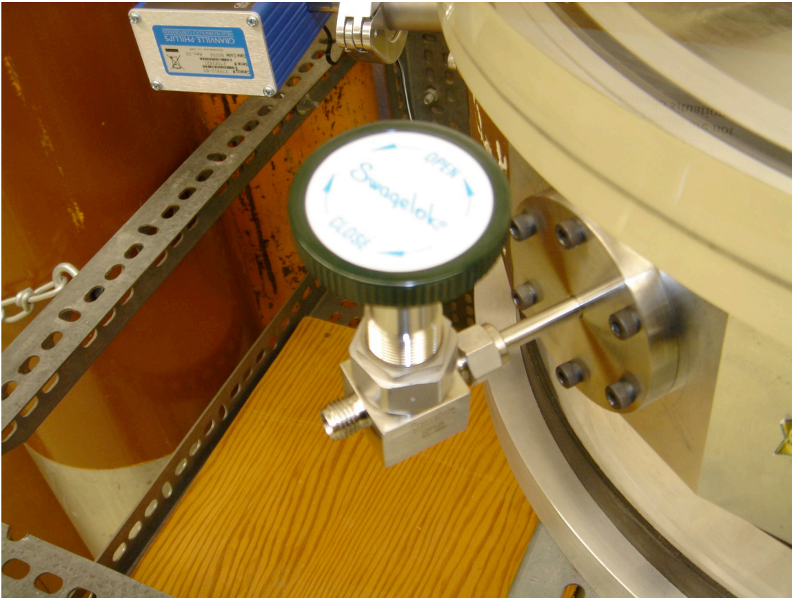
[Fig. 14]: Swagelok bellows valve to vent test chamber back to atmospheric pressure. (Teflon tubing not pictured.)
