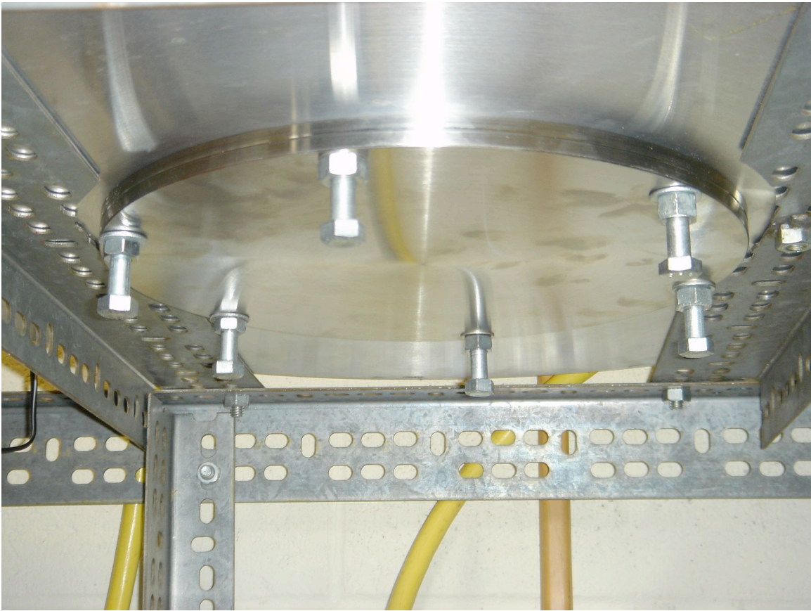
[Fig. 13]: Custom stainless steel plate to cover exposed hole in test chamber.
