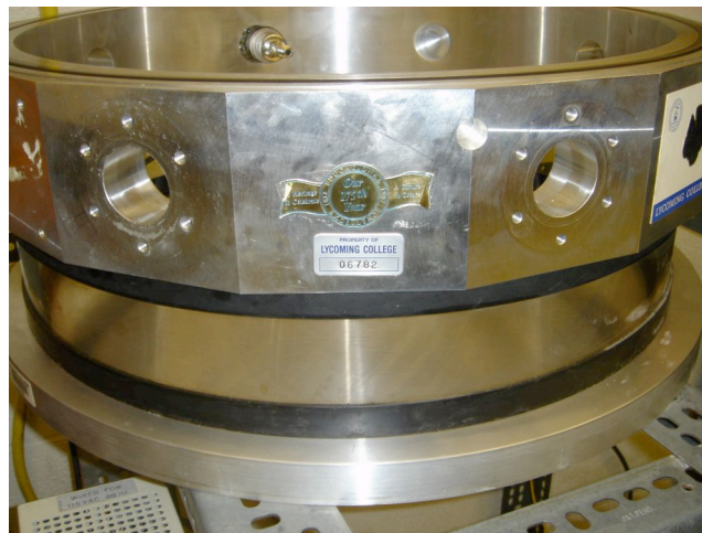
[Fig. 4b]: Chamber collar, glass cylinder, and stainless steel plate.
