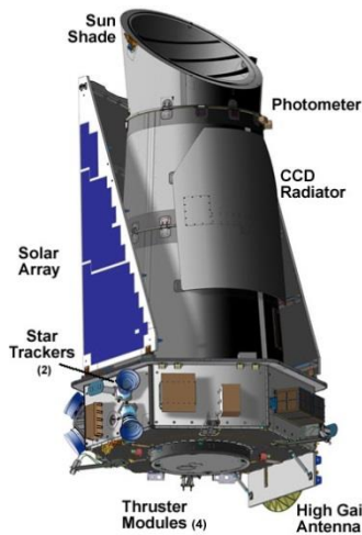
Figure 4a (left): Diagram of Kepler Spacecraft and its components including the Photometer.
